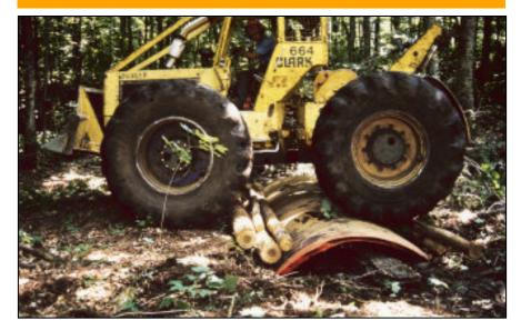
rotecting water and stream environments is important to the forest industry. To do so, safe, reliable and affordable water crossings are required. These crossings, or arches as they are called, allow crossed streams to remain undisturbed.
